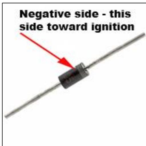
Make sure you reference the "line" on the diode in the right orientation. The line denotes the cathode or the "negative" side. You want this cathode line facing the ignition.....the side without the line going to the battery or supply voltage.
